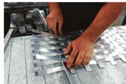
Aluminum woven components are constructed by weaving various widths of aluminum strips by hand for a traditional wicker effect.
